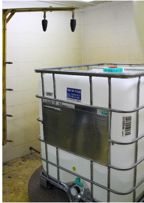
Photos of rinsing station inside our warehouse. Plastic covers were pulled back for photo purposes, and the tank in the photo held only water.
